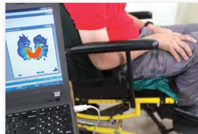
運用電腦系統能準確檢測服務使用者腰背的壓力分佈，從而揀選合適的減壓座墊，提升承托力及舒適度。 Computerised system was used to accurately gauge pressure distribution on the back, in order to choose the appropriate pressure-relieving cushions for greater support and comfort.
