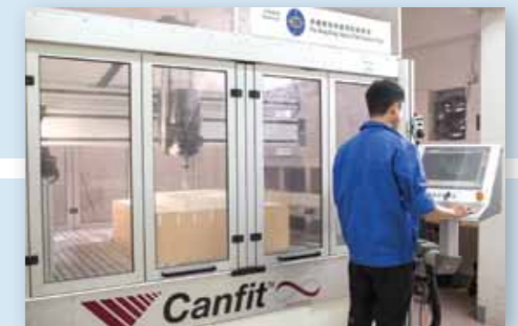
中心利用「電腦輔助設計製造系統」製作個人化塑形座椅，系統的自動磨刀會按三維立體掃描影像，刨挖出座椅墊，再經加工後便可安裝於輪椅上。 JCRSSC used "Computer-aided Design and Manufacturing System" to produce personalised sculpted seating. The system's automatic sharpener would scoop out the cushion in accordance with the body 3D scan. It would be fitted on a wheelchair after processing.
